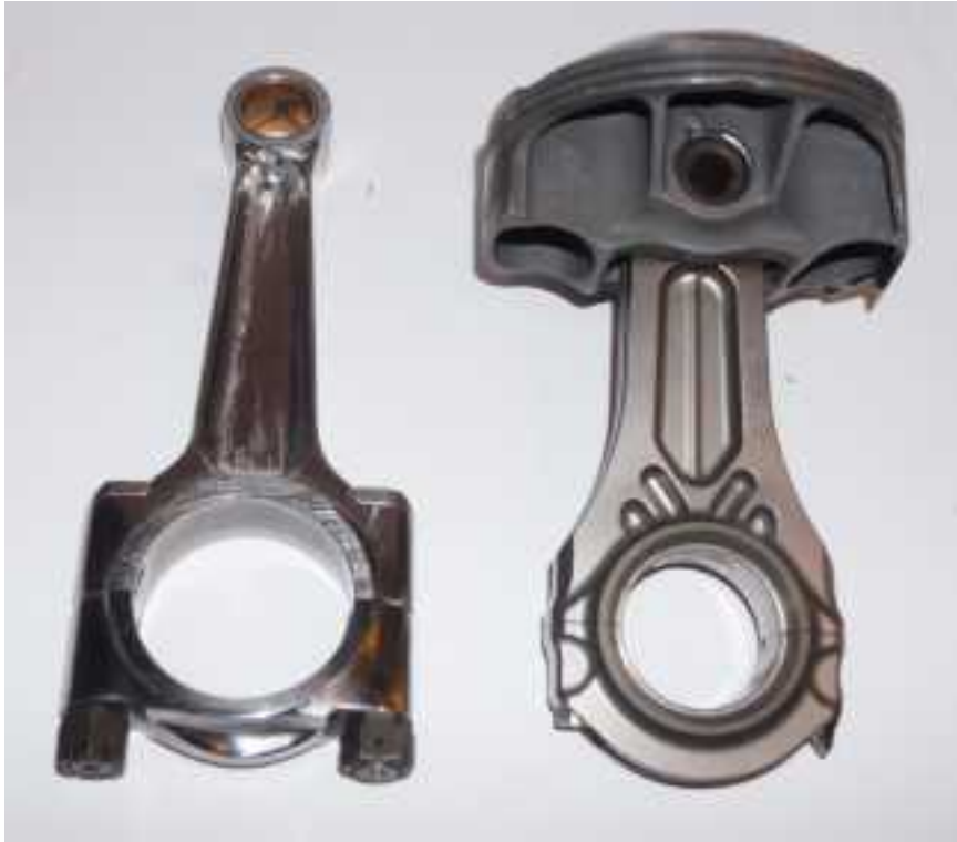
RODS from Ferrari, GTO 1963 left and 2004 F1.
